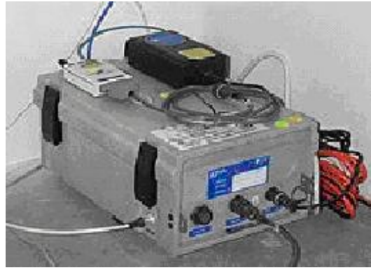
Figure 6.1: This is a photo of a seismometer used to measure the magnitude and location of earthquakes.
