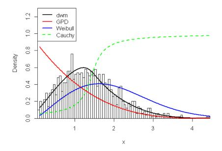
Figure 8: Example of simulated Weibull data with overlaid fitted dynamic weighted mixture model.
